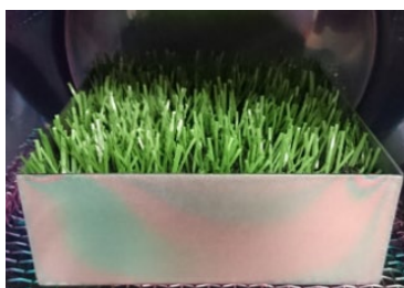
Figure D-1. Example of a 6 x 6 x 2 inch reconstructed turf field sample for emission testing
