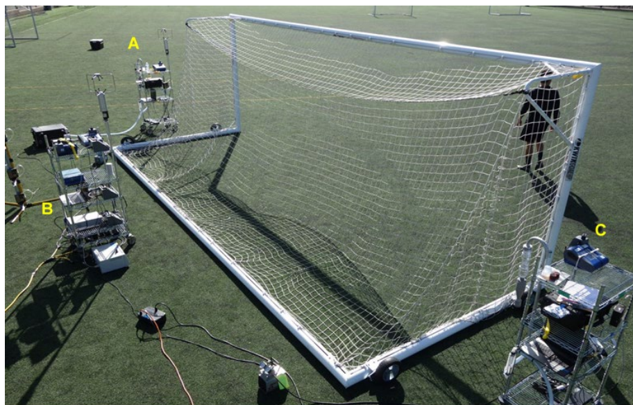
Figure 2-1. Volatile Compound Sampling Packages A: Cart 1, on field at the right side of the monitoring unit (white goal box). B: Cart 2, on field at the back of the monitoring unit. C: Cart 3, on field at the left side of the monitoring unit. Each package was positioned 1 meter above the field surface.
