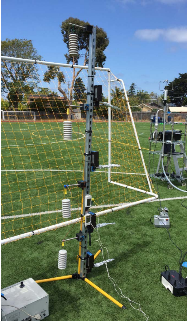
Meteorology and VOC stratification tower
